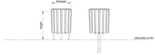
**Dimensions** Diameter - 457mm, height - 570mm excluding fixings. (sizes are approximate)
