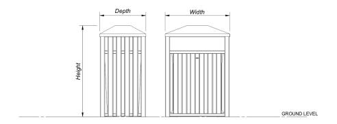
**Dimensions** Width - 695mm, depth - 495mm, height - 987mm. (sizes are approximate)
