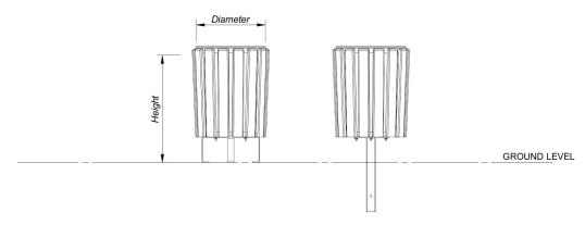
**Dimensions** Diameter - 457mm, height - 570mm excluding fixings. (sizes are approximate)
