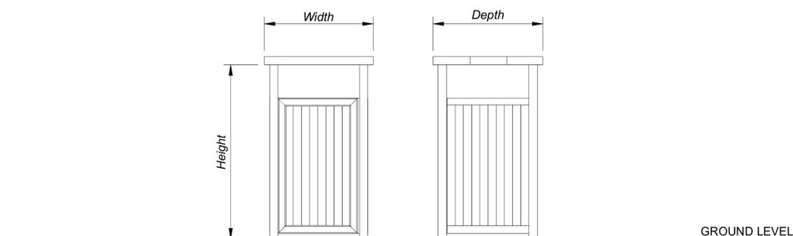
**Dimensions** Width - 580mm, depth - 580mm, height - 950mm. (sizes are approximate)
